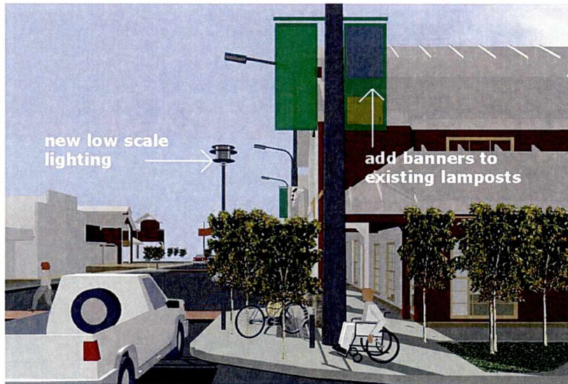
Public lighting and street furniture - low scale lighting units that add onto or replace existing light standards / add banners to lamp posts
